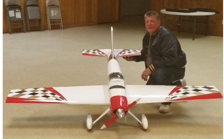
Brian applied the monokote checkering with NO-HEAT Trim Solvent. (photo from Bill Froeder)
