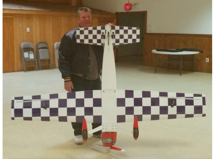
Brian applied the monokote checkering with NO-HEAT Trim Solvent. (photo from Bill Froeder)
