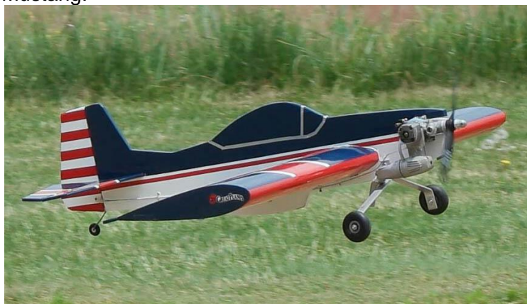
Sheldon Parker's kit built 44", OS 46-powered profile Mustang.
