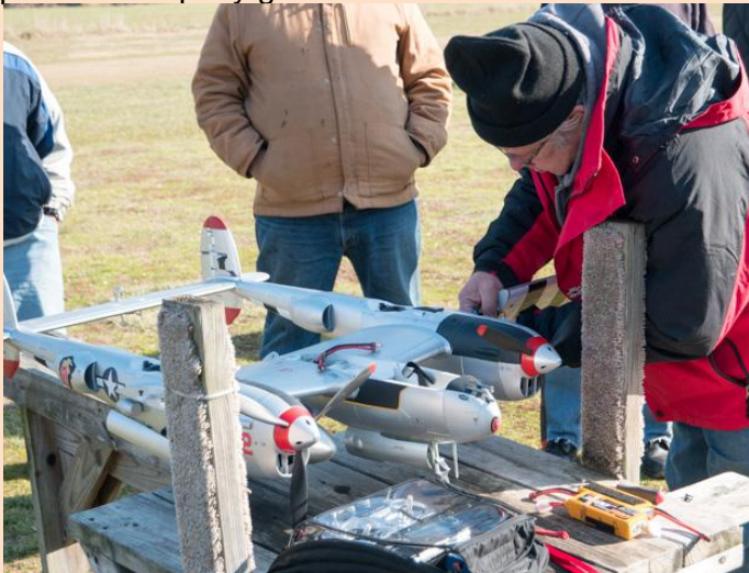
Gregg Clement setting up his Motion RC, foam, 63" P-38L Lightning. The "fork tailed devil" came as a PNP complete with pre-installed retracts, sequenced gear doors, flaps, LEDs, servos, brushless motors and with a set of 3-blade and a set of 2-blade counter-rotating props. Gregg said he was very happy with the parts support the company gave him.
